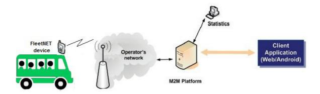
The back-end server is cloud based and does not require any installation or maintenance by the customer. The FleetNET management application is available via any web browser, from any computer connected to Internet.
